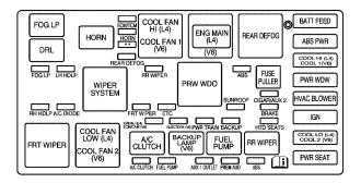
The underhood fuse block is located in the forward part of the engine compartment near the battery.
